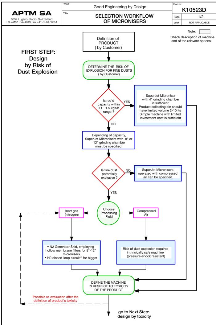
Note: The choice of Nitrogen-inerted systems can be determined by the construction of machine in respect to the product toxicity. Nitrogen generator skids are strongly recommended for toxic products, where Isopak-series must be employed
