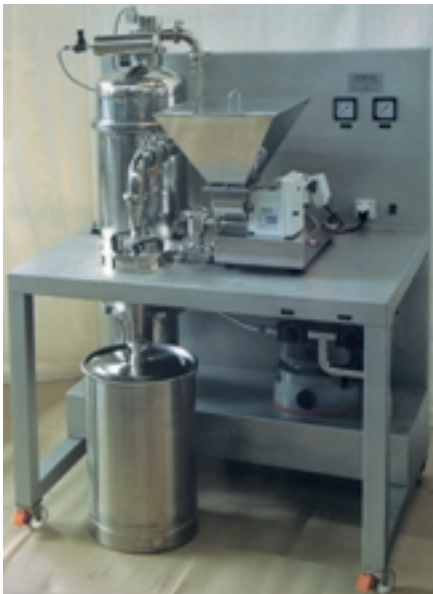
SUPERJET KOMPAK-2, OPERATED WITH COMPRESSED NITROGEN
