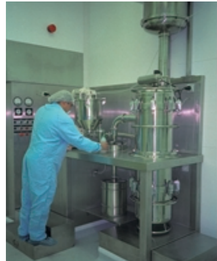
N 2 -INERTED SYSTEM, CLASS 1000 ENVIRONMENT
